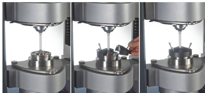
Fig. 4: Parallel plate geometry in measurement position without and with sample cover.
