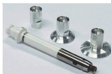
Fig. 5: Adapter for disposable plates with plate inserts of different diameters.
