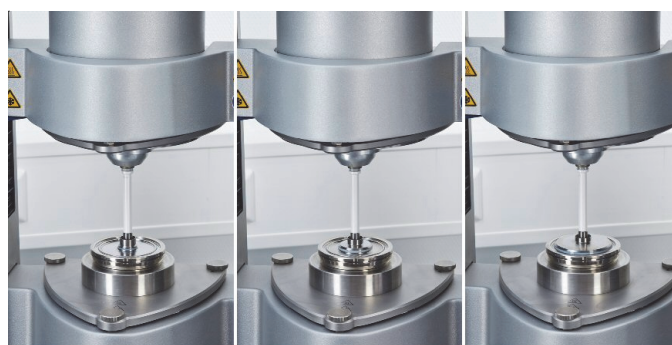
Fig. 2: Selection of parallel plates geometries with different diameters (20 mm, 35 mm and 60 mm).
