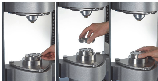
Fig. 1: Mounting of a lower plate on top of a temperature module.
