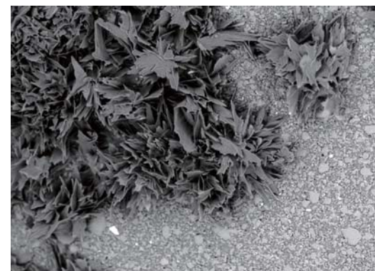
TM4000 5kV 5.9mm X300 BSE M Accelerating voltage: 5 kV Image signal: BSE Magnification: 500x Sample: Chocolate Cooling stage used
