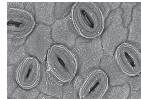
TM4000 10kV 5.8mm X1.00k BSE H Accelerating voltage: 10 kV Image signal: BSE Magnification: 1,000x Sample: Leaf stomata
