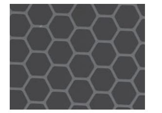
Hexagonal support grid for increased transmission
